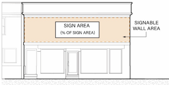
Example of signable wall area
